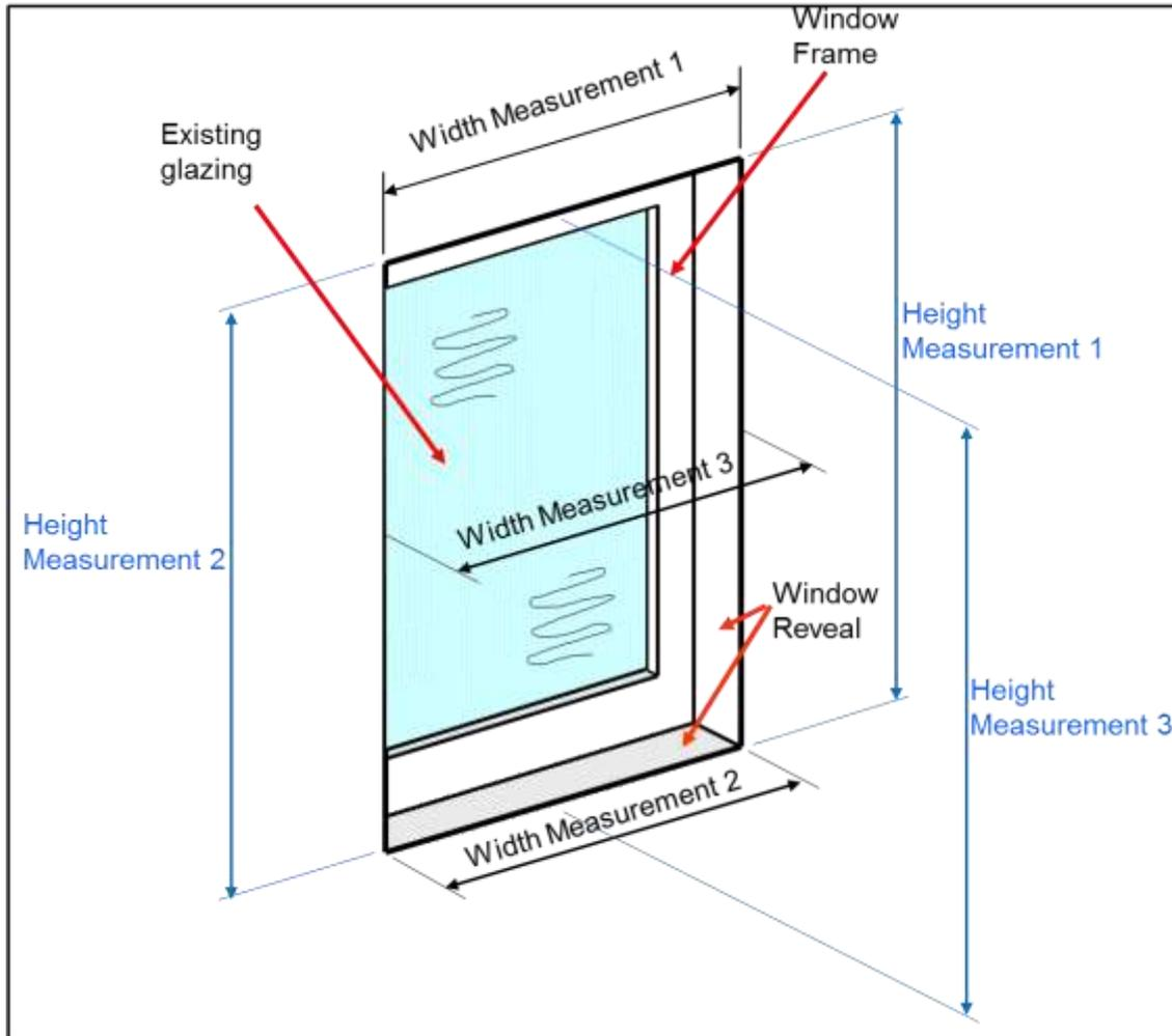
**Recommended steps to measure your existing window reveal to identify your window reveal height and width.**
